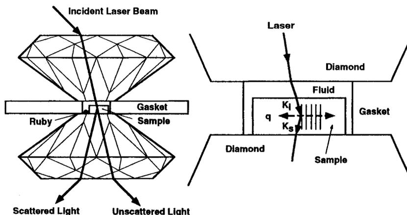
**Figure 1.** Brillouin scattering in the diamond anvil cell. Wavevectors for the incident photon ( $k_i$ ), scattered photon ( $k_s$ ), and phonon ( $q$ ) are shown at the right. In the platelet geometry, light enters and exits the sample from opposite, parallel faces, and the acoustic wave propagates in the plane of the sample.
