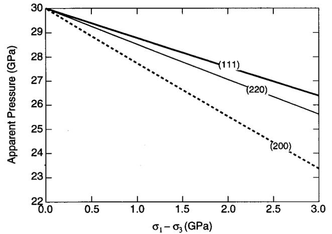
FIG. 5. The apparent pressure determined by assuming the measured  $d$  spacing for the (111), (200), and (220) diffraction lines of platinum correspond to the volume strain under hydrostatic pressure, as a function of differential stress,  $(\sigma_1 - \sigma_3)$ . The hydrostatic pressure is 30 GPa.
