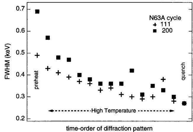
FIG. 8. Platinum diffraction line width for N63A. The FWHM of platinum diffraction lines (111) (+) and (200) (■) plotted in order of measurement.
