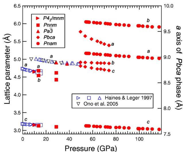
FIG. 2. (Color online) Variation of lattice parameters of SnO<sub>2</sub> phases as a function of pressure. The solid symbols are from this study; open symbols are from previous reports (Ref. 5,7). The  $Pa\bar{3}$  data of Ref. 7 are shown with a down pointing triangle to distinguish them from the results of Ref. 5. Data obtained from  $P4_2/mnm$ ,  $Pnnm$ ,  $Pa\bar{3}$ , and  $Pbca$  phases were without heating, whereas those of  $Pnam$  phase were obtained after heating.
