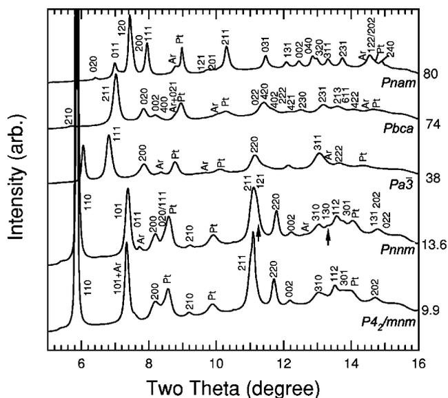
FIG. 1. Representative diffraction patterns for phases of  $\text{SnO}_2$  observed in this study. Each trace is labeled with pressure (in GPa) and space group of corresponding structure. The abbreviations are Pt for platinum and Ar for argon. The arrows emphasize the splitting of peaks from  $P4_2/mnm$  to  $Pnmm$ .
