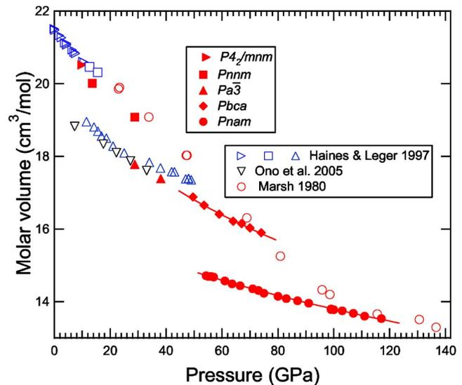
FIG. 4. (Color online) The molar volume as a function of pressure for SnO<sub>2</sub> phases at pressure to 117 GPa. The symbols used here are same as Fig. 2, except for open circles which represent shock compression data from Marsh (Ref. 22). Solid lines are second-order Birch-Murnaghan equation fits to *Pbca* and *Pnam* phase data. The *Pa3̄* data of Ref. 7 are shown with a down pointing triangle to distinguish them from the results of Ref. 5.
