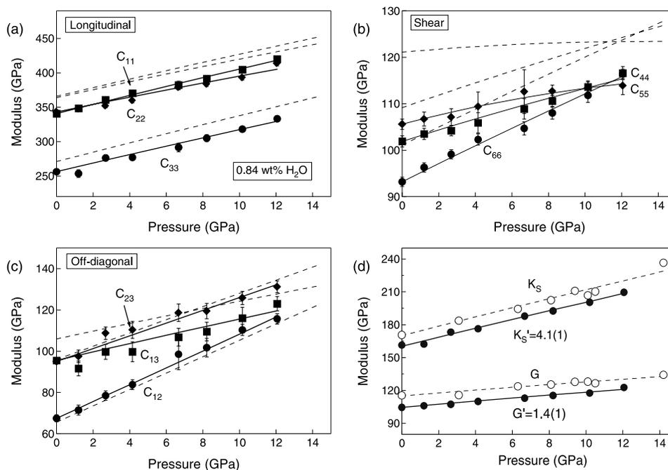
**Figure 1.** Elastic moduli of hydrous wadsleyite as a function of pressure compared with those of anhydrous wadsleyite [Zha *et al.*, 1997]. Solid symbols and lines: wadsleyite with 0.84 wt.% H<sub>2</sub>O, (this study); dashed lines: anhydrous wadsleyite, [Zha *et al.*, 1997]. (a–c) Individual  $C_{ij}$  of hydrous wadsleyite; (d) adiabatic bulk,  $K_S$ , and shear moduli,  $G$ .
