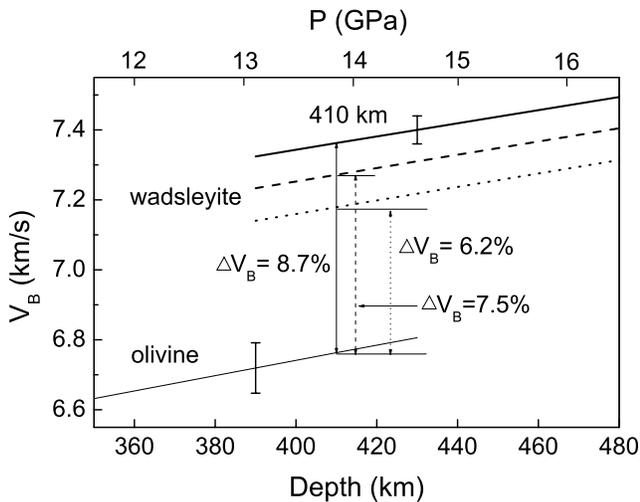
**Figure 2.** Bulk sound velocity as a function of depth along a mantle adiabat for anhydrous olivine and wadsleyite with variable hydrogen content. Pressure converted to depth using Earth model PREM [Dziewonski and Anderson, 1981]. Solid line: dry conditions; dashed line: 0.4 wt% H<sub>2</sub>O in wadsleyite; dotted line: 0.8 wt% H<sub>2</sub>O in wadsleyite. Representative uncertainties of the calculation are also shown.
