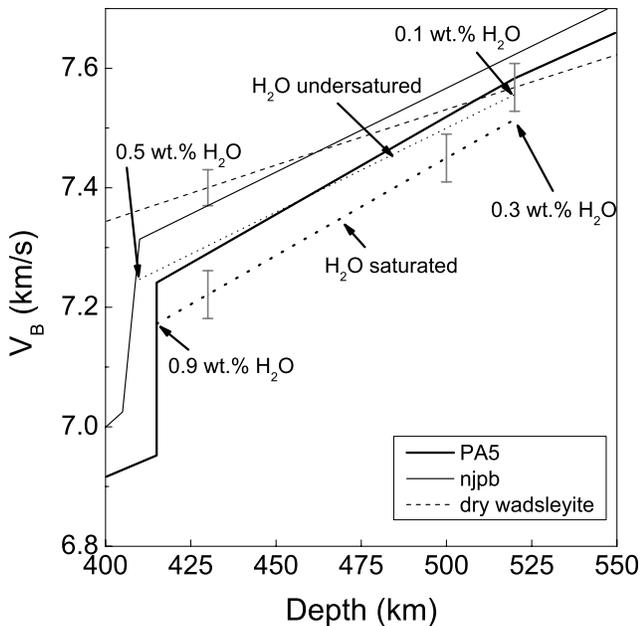
**Figure 3.** Effect of changes in H<sub>2</sub>O content on seismic gradient in the upper part of the transition zone. Seismic model PA5 and njpb are shown as solid lines. Dashed line: anhydrous wadsleyite; bold dotted line: H<sub>2</sub>O gradient under water saturated conditions; light dotted line: H<sub>2</sub>O decreases from 0.5 wt.% to 0.1 wt.%. Uncertainties of the calculation are also shown.
