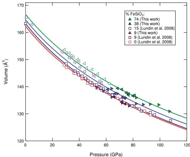
**Fig. 7.** Unit cell volumes measured on compression (right-pointing triangles) and decompression (left-pointing triangles) for (Mg,Fe)SiO<sub>3</sub> perovskites and Birch–Murnaghan equation of state fits. Open triangles were not used for equation of state fits due to significant deviatoric stresses. Volumes indicated by open squares are from Lundin et al. (2008). Pressures for this and previous work were determined by Au scale of Fei et al. (2007).
