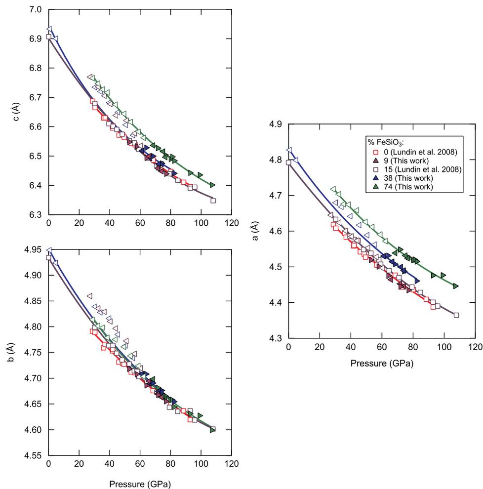
**Fig. 6.** Lattice parameters  $a$ ,  $b$  and  $c$  for perovskites measured upon compression (right-pointing triangles) and decompression (left-pointing triangles) compared with previous work (Lundin et al., 2008). Open triangles: data not used in equation of state fit due to deviatoric stress.
