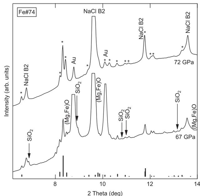
**Fig. 3.** Selected diffraction patterns for Fe#74 perovskite showing transition from perovskite to perovskite plus oxide mixture on decompression. Orthorhombic GdFeO<sub>3</sub>-type perovskite peaks are marked with asterisks and reference pattern is below. At 72 GPa, all peaks can be indexed to perovskite, NaCl medium or Au calibrant, but after heating at 67 GPa, CaCl<sub>2</sub>-type SiO<sub>2</sub> and (Mg,Fe)O peaks are also observed.  $\lambda = 0.3344 \text{ \AA}$  for these experiments.
