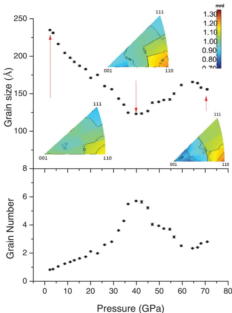
**Figure 7.** (Upper panel) evolution of the average size of the nano-domains determined from MAUD fits as a function of pressure. The inset shows the evolution of the domain/grain orientation of Au nanocrystallinity. (Lower panel) evolution of the number of nano-domains with pressure, suggesting an octahedron of six domains formed at 40 GPa.
