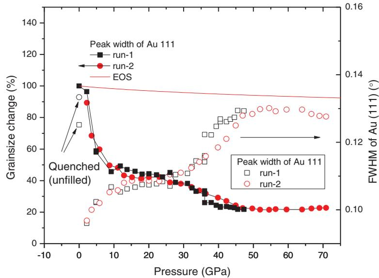
**Figure 5.** (Right axis) full width at half maximum (FWHM) of the Au 111 diffraction peak; (Left axis) percentage of original grain size as a function of pressure based on peak-broadening analysis. The unfilled square and circle indicate data on pressure release.
