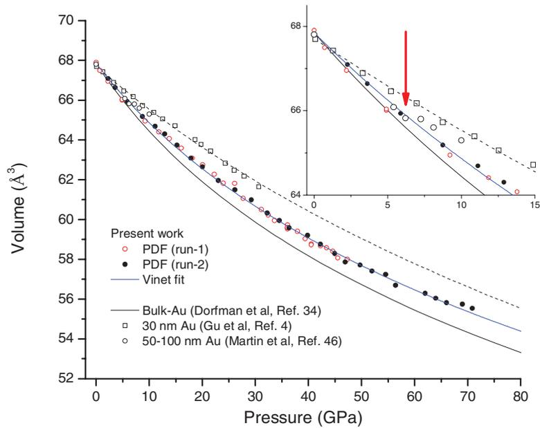
**Figure 3.** Pressure dependence of the unit cell volume of n-Au compared to previously reported data for 300 nm Au (dashed line) [4] and the bulk material (solid line) [34]. Vinet EOS fit is shown for the PDF data of run-1 and run-2. Inset shows an expanded view of the region at low pressure.
