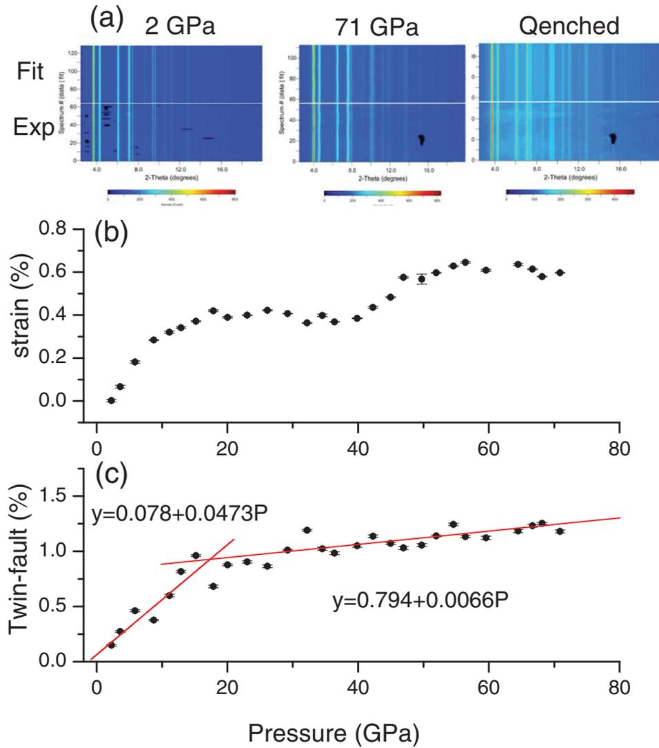
**Figure 6.** (a) Full-profile refinement for azimuthally (0 to 360°) unrolled diffraction images of n-Au (above: fit, below: binned data). (b) Evolutions of microstrain and (c) twin-fault probabilities refined by MAUD as a function of pressure, showing a turning point at 17.5 GPa and a factor of approximately seven-fold reduction in twin-fault probabilities.
