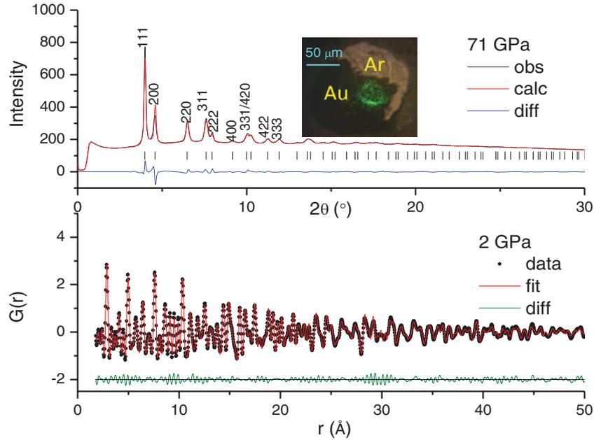
**Figure 2.** (Upper panel) Rietveld refinements of the diffraction patterns of n-Au at 71 GPa using Jana2006 software [53]. The inset shows an image of the gold samples (dark field) suspended in Ar pressure medium (bright field) illuminated by a green laser used for pressure measurement. (Lower panel) high pressure PDF fit for n-Au at 2.1 GPa with a fit residual,  $R_w$ , of 0.167.
