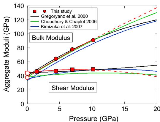
**Fig. 3** Aggregate bulk and shear moduli (Voigt-Reuss-Hill) of  $\alpha$ -quartz as a function of pressure. Filled red symbols are from this study with red line showing finite-strain fit (solid) extrapolated to 20 GPa (dashed). Ambient measurements (open red circles) are from (Every and McCurdy 1992). Black lines are from a previous high-pressure Brillouin study (Gregoryanz et al. 2000), green and blue lines are from theoretical studies (Choudhury and Chaplot 2006; Kimizuka et al. 2007)
