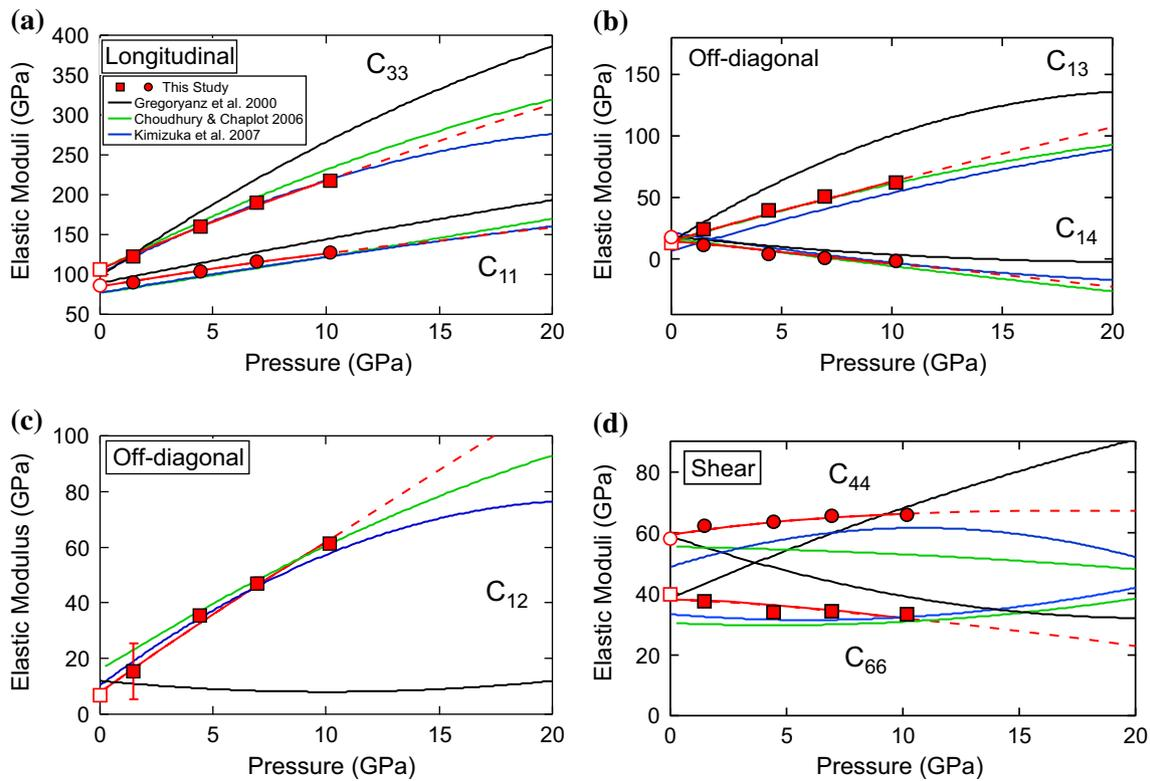
**Fig. 2 a–d** Elastic constants of  $\alpha$ -quartz as a function of pressure. Filled red symbols are from this study, and red lines are third-order finite-strain equation fits (solid) extrapolated to 20 GPa (dashed). Data at ambient conditions (open red symbols) are from an average of previous studies reported in (Every and McCurdy 1992). Black lines
